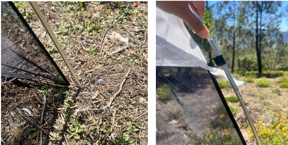
Figure 4. Metal stack/peg placed at one of the extremes of the Malaise trap (left). Gray tape placed in the joints of the trap metal structure for reinforcement (right).
