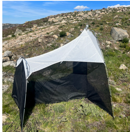
Figure 1. Scheme of a Townes Style Malaise trap used in the present study and its approximate dimensions (left); and example of a Malaise trap set in Serra da Estrela, Portugal (right).
