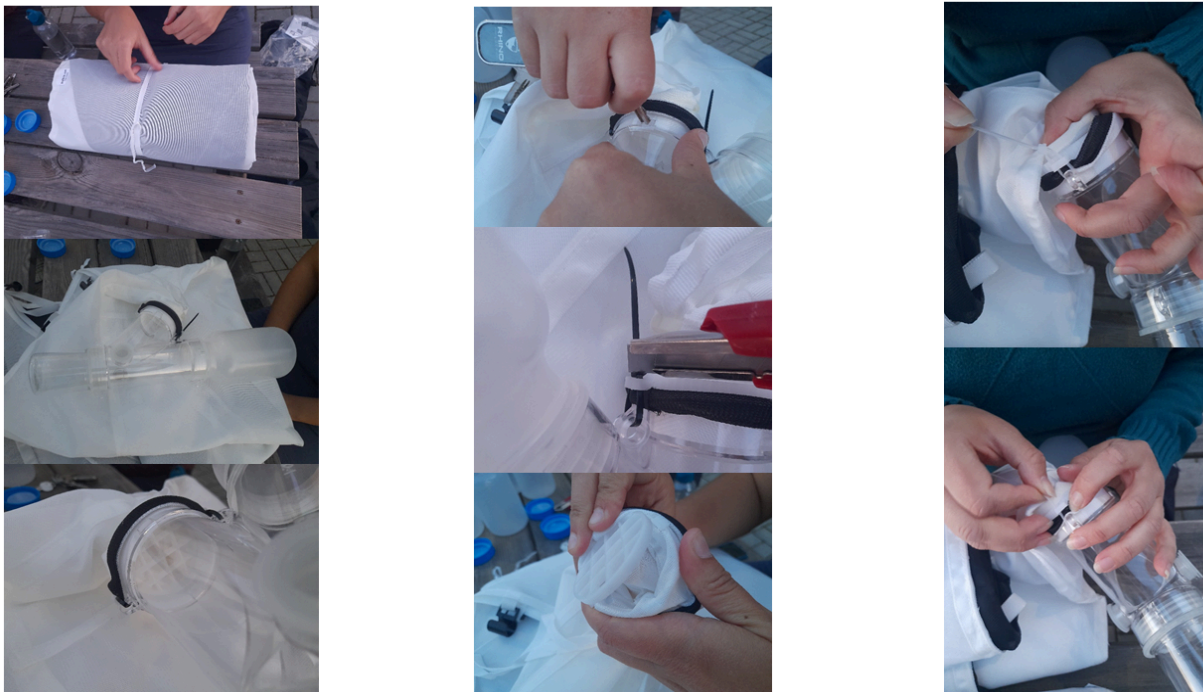
Figure 3. Example of how to remove the plastic grid included in the Malaise trap.
